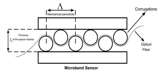
Intensity modulation caused by microbending in multimode fibers can be exploited as a transduction mechanism for detecting environmental changes. The change in light transmission,  $\Delta T$ , through a microbend sensor can be formulated as:
