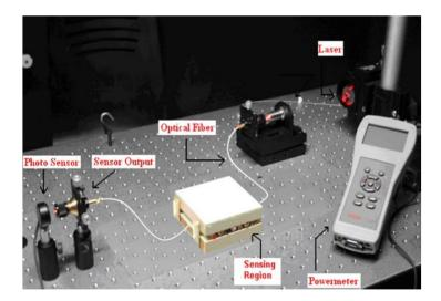
Figure 4 shows the results obtained from this experiment. From this figure it can be observed that as the applied force increases, the output light intensity decreases. The amount of light loss while increasing the force is an important parameter for sensitivity in fiber optic microbend sensors since the magnitude of the measurand can be determined by correlating the loss of light intensity.
