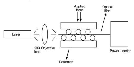
Figure 3. Experimental setup.
