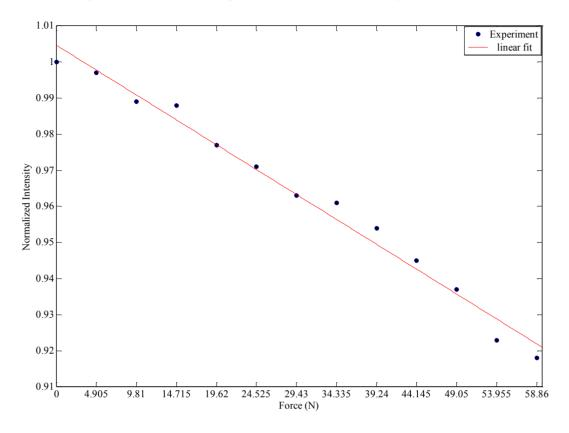
Figure 4. The sensor response (normalized intensity) in terms of F.
