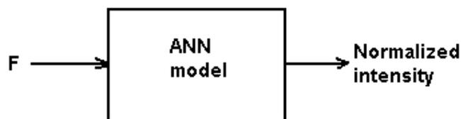
F is a known parameter and can be utilized for the prediction of the sensor response. A training dataset consisted of randomly selected F vs. normalized intensity is exploited to the network and the network is trained. After the training process, new responses are predicted for unseen F values.
