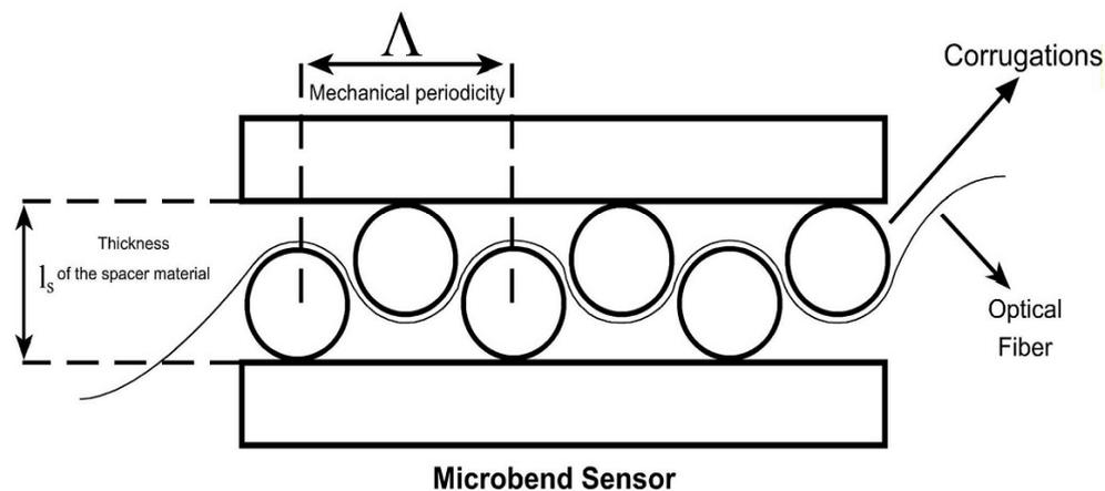
Intensity modulation caused by microbending in multimode fibers can be exploited as a transduction mechanism for detecting environmental changes. The change in light transmission,  $\Delta T$ , through a microbend sensor can be formulated as:
