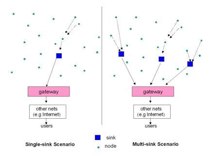
Figure 1. Left part: single-sink WSN. Right part: multi-sink scenario.
