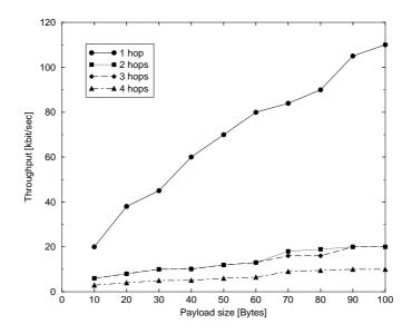
In Figure 12 a single-sink scenario where 802.15.4 nodes transmit data to the sink through one link (star topology), or possibly two-hops (3-level tree, rooted at the sink), is considered. A network composed of 30 nodes, working in beacon-enabled mode is accounted for. In the figure we show the throughput as a function of the size of the packets transmitted by nodes. The throughput here represents
