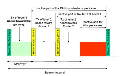
Figure 10. The superframe structure used in the tree-based topology.
