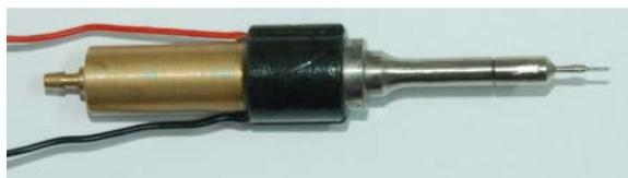
Based on the above calculations, an ultrasonic probe with a nano tungsten needle was fabricated as shown in Figure 8. The cell penetration experiments were done using this probe.
