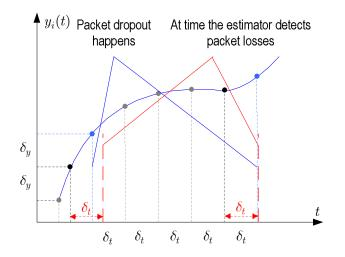
Figure 2. Multiple packet dropout detection.
