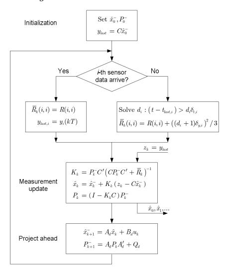
Figure 4. Structure of the modified Kalman filter.
