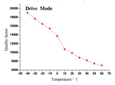
Figure 6. Trend of quality factor change with temperature in drive mode.
