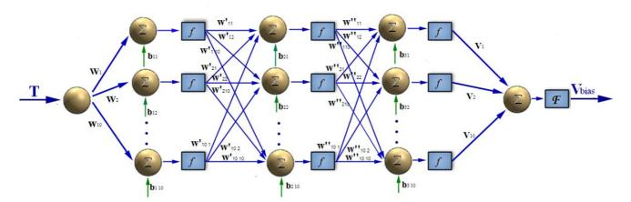
Figure 14. Structure of the BP neural network adopted for modeling.
