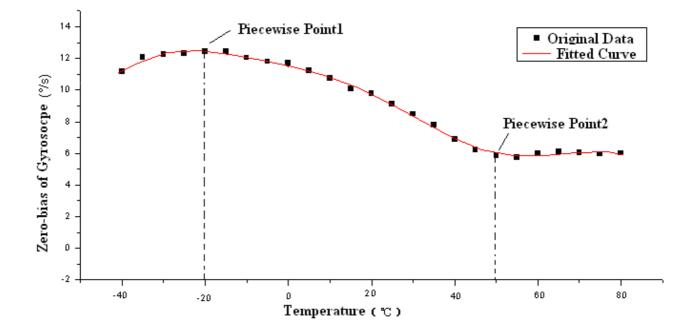
Figure 18. Fitted curve of zero bias of microgyroscope with temperature.
