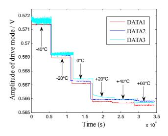
Figure 11. Trend of drive amplitude change with temperature.
