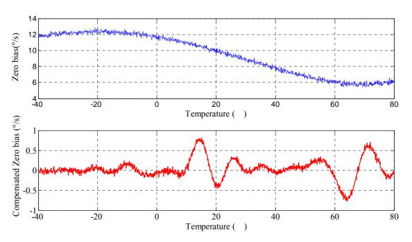
Figure 17. Verification of BP neural networks compensation effects.
