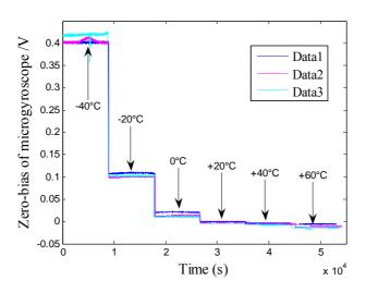
Figure 12. Closed-loop test of zero bias of microscope with temperature changes.
