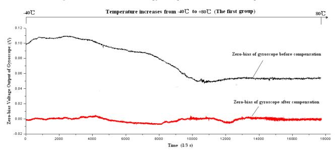
Figure 20. Zero bias of microgyroscope before and after compensation.
