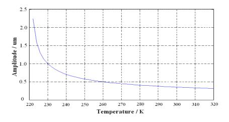
Figure 3. Simulation of relationship between the output amplitude and the temperature.
