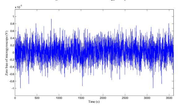
Figure 27. Zero bias of Microgyrosope.
