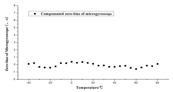
Figure 23. Compensated zero bias of the microgyroscope.
