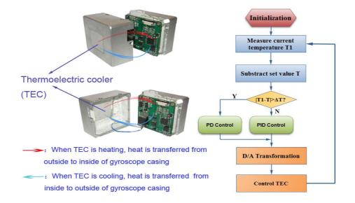
Figure 25. Gyroscope casing design and system software flow chart.
