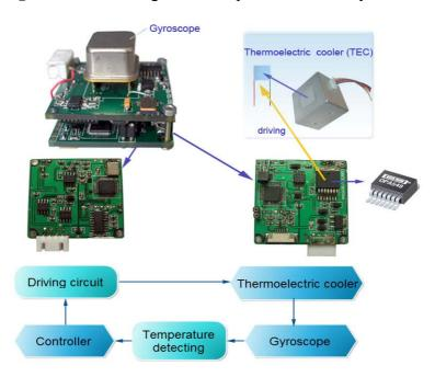
Figure 24. Block diagram of temperature control system.
