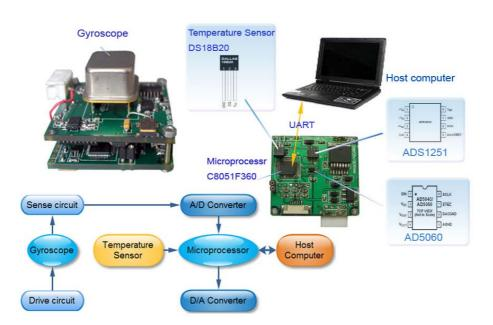
Figure 19. Diagram of the temperature compensation system.
