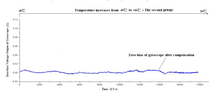
Figure 21. Zero bias of microgyroscope after compensation.
