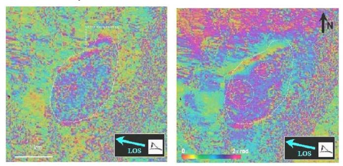
The dotted circles on Figure 2 left show areas that seem to move slightly faster (along the LOS) than the rest of the landslide. The white frame in the north east of the landslide points a fringe pattern that is not confirmed on the right image. It could be a displacement which occurred during the period 02/01/1997-15/02/1997. The observed signatures correspond to less than three fringes. An
