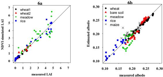
For LAI estimation, the best fitted values found for  $NDVI_{\infty}$ ,  $NDVI_{s}$ , and  $K_{LAI}$  were respectively 0.9, 0.1, and 0.70, with a RMSE<sub>R</sub> of 26.8%. The results compared to ground measurements were globally satisfactory as displayed in figure 6a. Those values were very comparable to those obtained in other studies [27, 35]. However, we can notice more dispersion for irrigated meadows at high LAI values.
