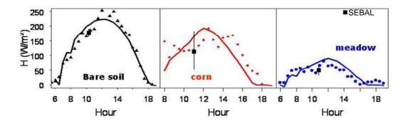
**Figure 9**. Sensible heat flux computed with the SEBAL model for the July 26 2006 at 11:30 TU, **a**) compared to the measurements performed over various fields, **b**) over a small area extracted from the FORMOSAT and FLIR images.
