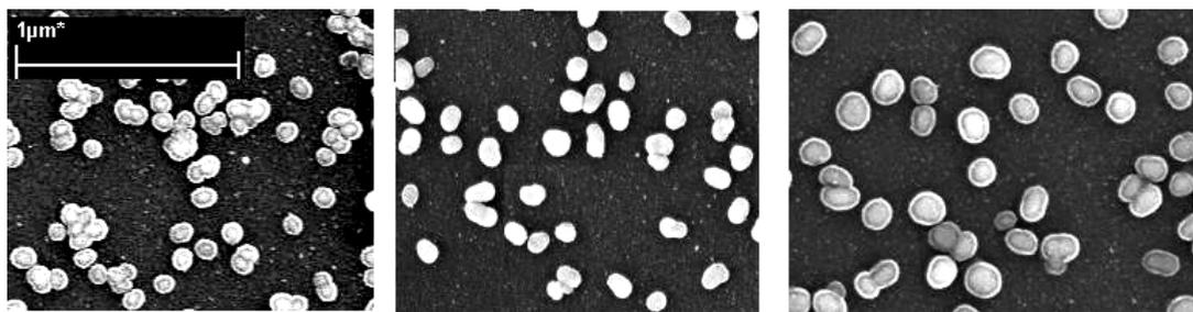
**Figure 7.** SEM images of (A) 80 nm Au colloid; (B) 118 nm Au colloid; (C) 162 nm Au colloid after 24 hours deposition onto the APTMS modified glass substrates. All images were taken at the same magnification (50K [15]). Reprint with permission from [15]. Copyright (2008) American Chemical Society.
