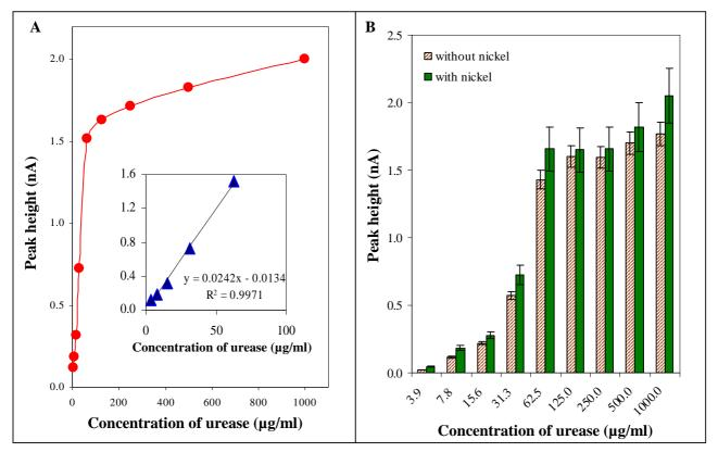
**Figure 6.** Dependence of urease peak height on its concentration within the range from 1 to 1,000  $\mu$ g/ml) and from 1 to 60  $\mu$ g/ml (**inset**) (**A**). The influence of nickel(II) ions on DPV urease signal (**B**).
