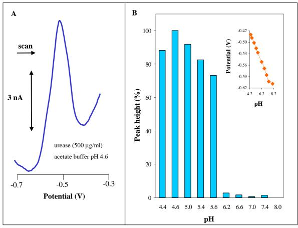
Figure 4. Differential pulse voltammogram of urease (500 μg/ml) measured in the presence of acetate buffer (0.2 M, pH 4.6) and accumulation time of 120 s (A). Changes in urease peak height in the presence of acetate (pH of 4.4 – 5.6) and phosphate buffer (pH of 6.2 – 8.0); in inset: the influence of pH on potential of the peak (B).
