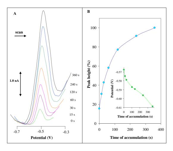
Figure 5. Typical DP voltammograms of urease (500 μg/ml) measured under various accumulation times (A). Dependences of urease peak height and its potential (in inset) on accumulation time (B). For other details see in Figure 4.
