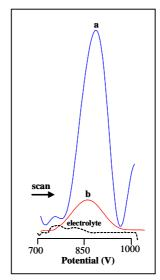
**Figure 8.** Square wave voltammetric analysis of urease using Ni nanoelectrode. The supporting electrolyte (acetate buffer pH 4.2) – dot-and-dash black curve, a) denatured urease (30 min, 99 °C), b) native urease. Concentration of urease (100 mg/ml). SWV parameters were as follows: frequency 200
