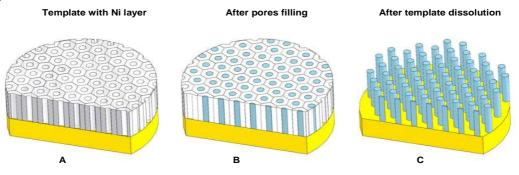
**Figure 1.** Whatman Anodisc as the template with sputtered Ni layer on the bottom (**A**), nanopores filled with Ni nanocrystal undergalvanostatic conditions (**B**), Ni nanopillars obtained after dissolution of the template (**C**).
