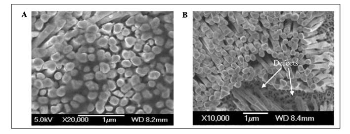
**Figure 7.** SEM analysis of Ni nanopillars created on the electrode, homogenously distributed Ni nanopillars (**A**) and detail of surface defects without Ni nanopillars (**B**).
