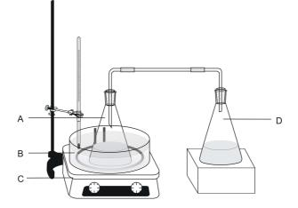
**Figure 1.** Apparatus for silver nanoparticles synthesis (A. conical flask with AgNO<sub>3</sub> solution; B. constant temperature water bath; C. magnetic stirrer; D. conical flask with NH<sub>3</sub>.H<sub>2</sub>O).
