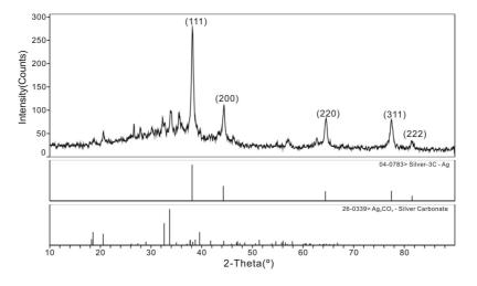
Figure 6. XRD pattern of the silver nanoparticles.
