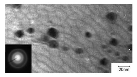
Figure 5. TEM image and the corresponding ED pattern (inset) of silver nanoparticles sample.
