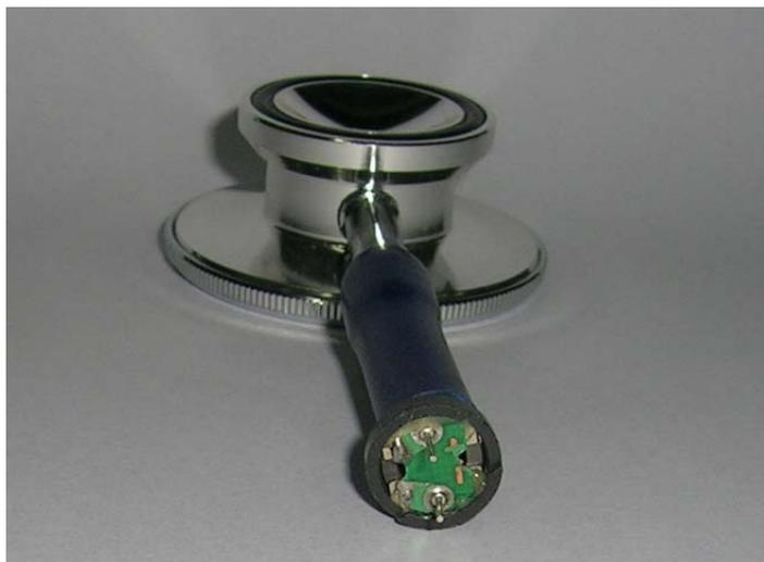
Figure 13. PZT is inserted in stethoscope.
