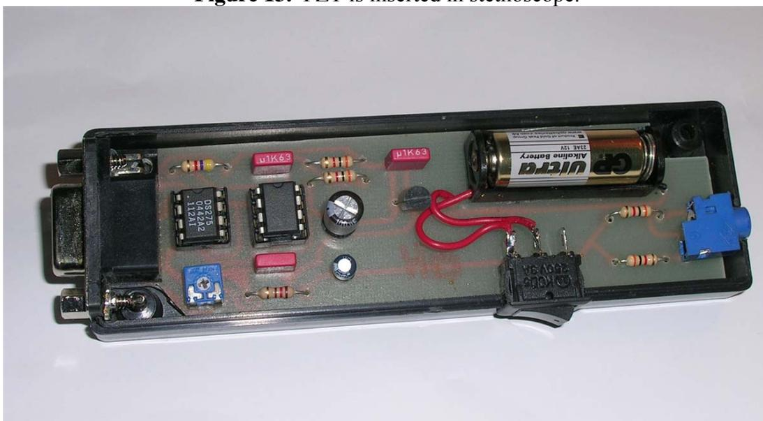
Figure 14. Prototype of aural vital signs system.
