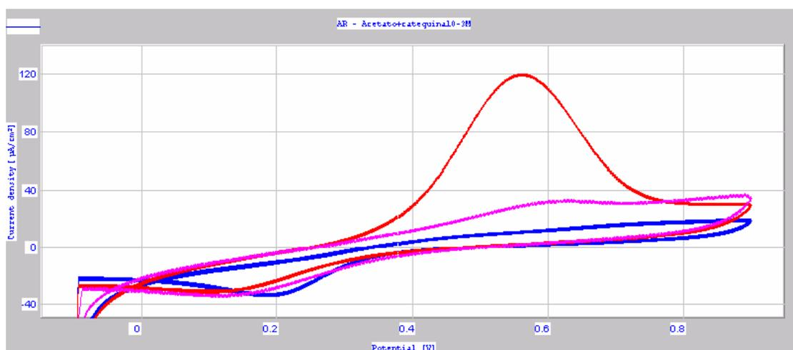
**Figure 4.** cyclic voltammograms of --Blue 1): (+)-catechin  $10^{-3} M$  in acetate buffer pH 4.5 (10mV/s); red 2) : (+)-catechin  $10^{-2} M$  in acetate buffer pH 4.5 (10mV/s); pink 3) (+)-catechin  $10^{-2} M$  in acetate buffer pH 4.5 (20mV/s).
