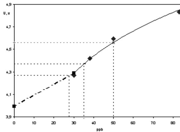
**Figure. 1** Ozone concentration dependence of sensor signal (Calibration curve).
