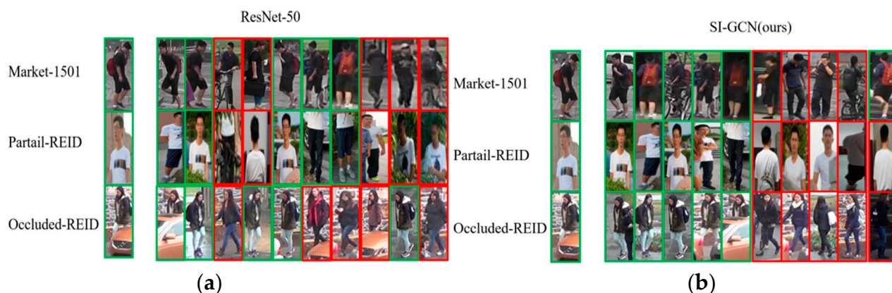
Figure 8. Qualitative comparison of top-10 ranking results between (a) the baseline and (b) SI-GCN on the Market-1501, Partial-REID and Occluded-REID datasets. Green boxes indicate correct matches, and red boxes indicate incorrect matches.
