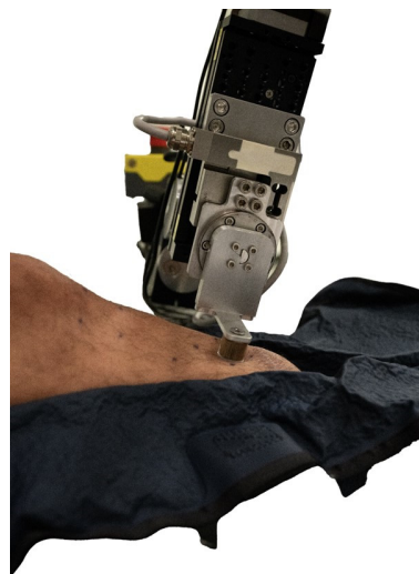
Figure 2. Load applicator aligned to participant's residual limb for load application. The leg is vacuum-splinted to stabilize the limb and limit motion during loading.
