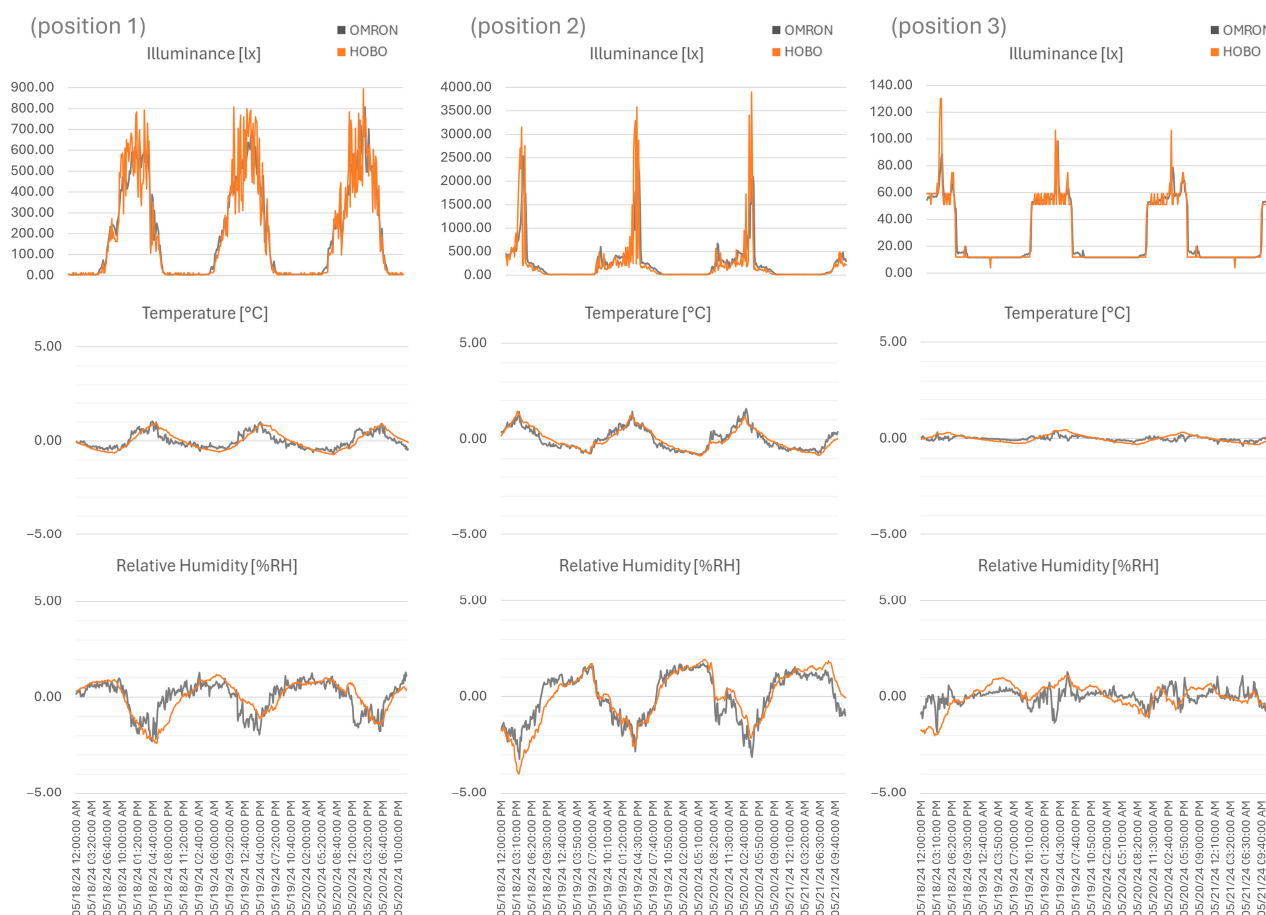
Figure 6. Illuminance (lx), temperature (°C), and relative humidity (% RH), from 18 to 20 May 2024, for HOBO and OMRON (average 10 min) for the three positions, synchronized by features and linear calibration (offset and gain correction).
