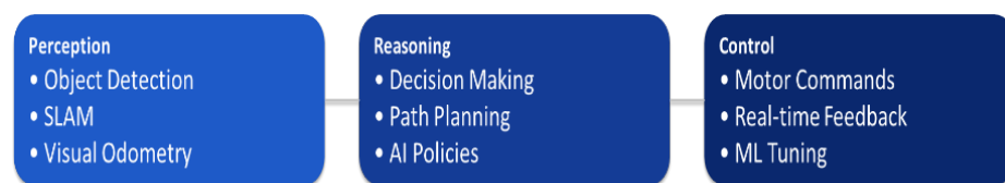
Figure 11. Layered autonomy architecture illustrating interactions among perception, mapping, planning, and execution modules in modern UGV systems.
