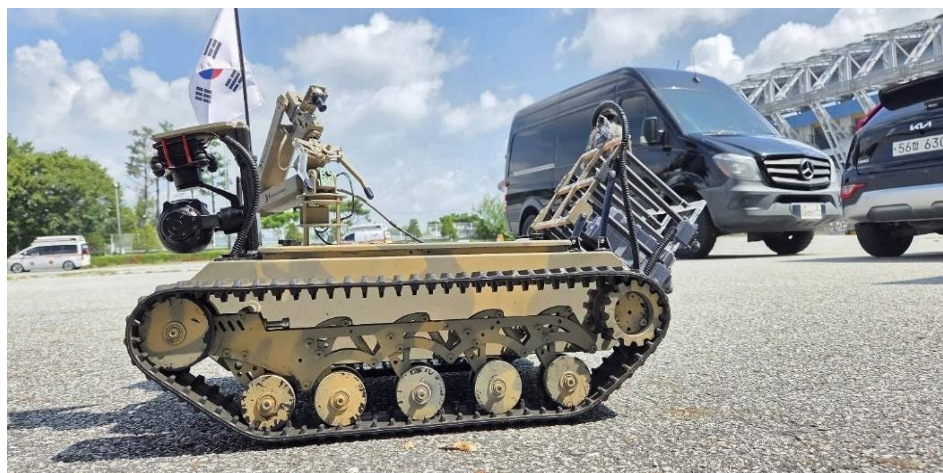
Figure 1. Representative unmanned ground vehicle (UGV) platform for disaster reconnaissance, illustrating the chassis structure, sensor placement, and mechanical configuration. The figure is provided for conceptual visualization only and does not report experimental results.
