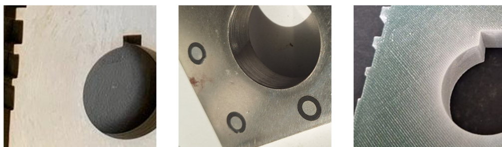
Figure 2. Evaluation of scanning performances under different surface scenarios. Example of the tested condition for the metal sample: raw surface without treatments ( left ), optical tracking markers ( center ), temporary matte scanning spray ( right ).
