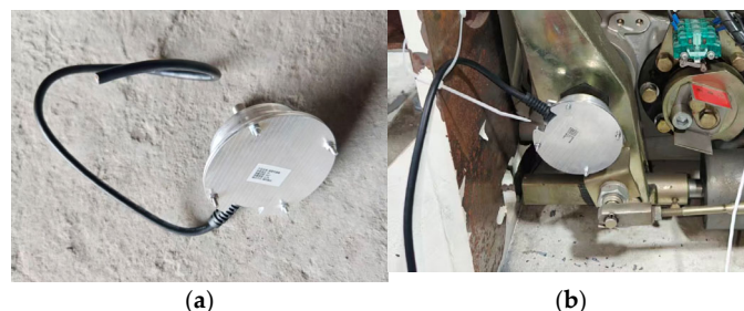
Figure 5. Opening/closing travel sensor: (a) physical sensor and (b) sensor assembly diagram.
