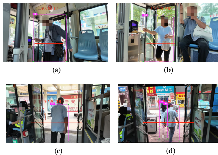
Figure 14. Public transport passenger flow statistics results (a) Boarding Passenger Flow Statistics (b) Boarding Passenger Flow Statistics (c) Alighting Passenger Flow Statistics (d) Alighting Passenger Flow Statistics.
