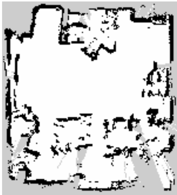
Figure 8. Occupancy grid map used in the narrow indoor environment with a resolution of 0.05 m.
