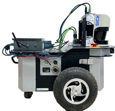
Figure 2. NRLAB02 differential-drive mobile robot platform equipped with a 2D LiDAR, inertial measurement unit, and wheel odometry sensors.
