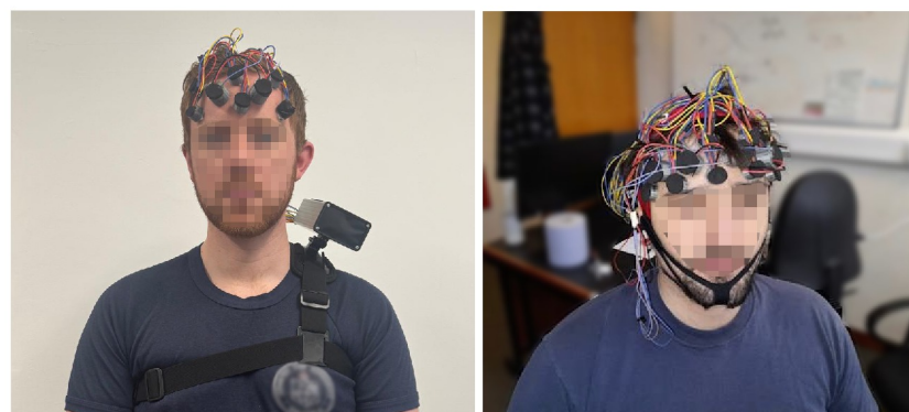
Figure 4. Wearable configurations of the proposed system. (Left): shoulder-mounted configuration during fNIRS-only operation. (Right): standard EEG cap configuration with fNIRS optodes positioned on the frontal scalp.
