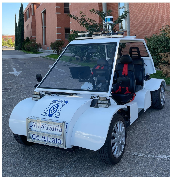
(c) Final vehicle with bodywork, drive-by-wire, HMI and sensor rack mounted on the roof
