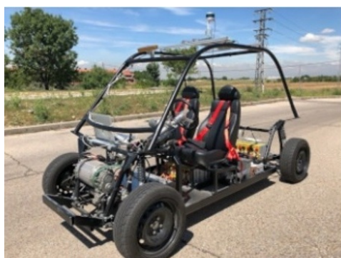
(b) Custom-designed tubular upper body, mounted on the base chassis
