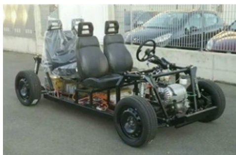
(a) Base chassis as purchased, including motor and batteries
