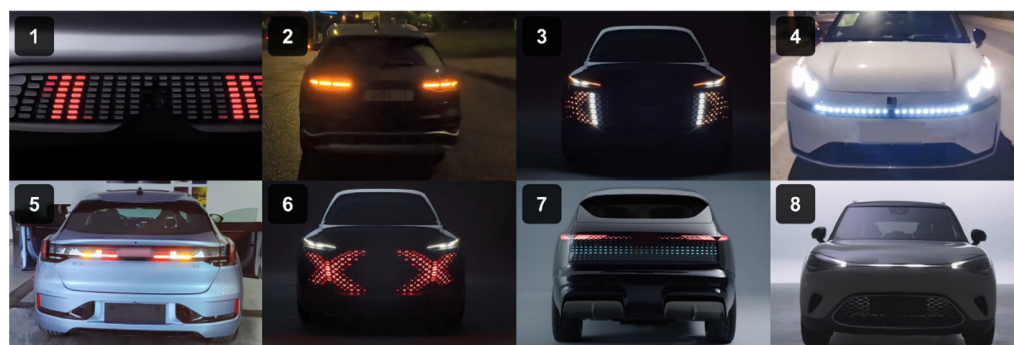
Figure 3. Eight eHMI types in real car design (No. 1: S-L-H; No. 2: S-S-H; No. 3: S-L-S; No. 4: S-S-S; No. 5: F-S-H; No. 6: F-L-H; No. 7: F-L-S; No. 8: F-S-S).
