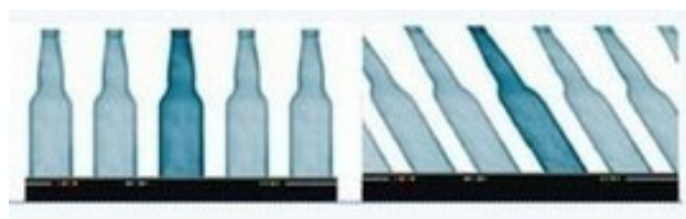
Figure 4. Rolling shutter effect diagram.
