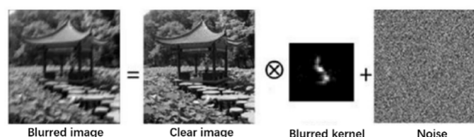
Figure 3. Fuzzy image formation process of motion blur diagram.
