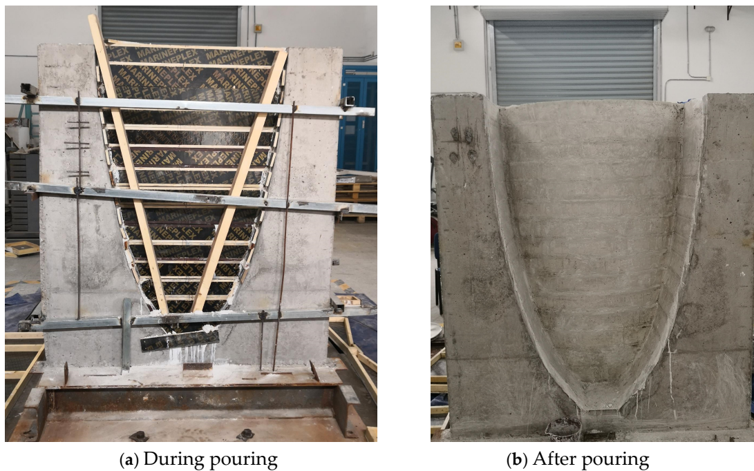
Figure 13. Physical model of the arch dam.
