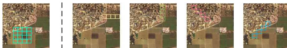
(a) Schematic diagram of capturing road information using square convolution and bar convolution in different directions
