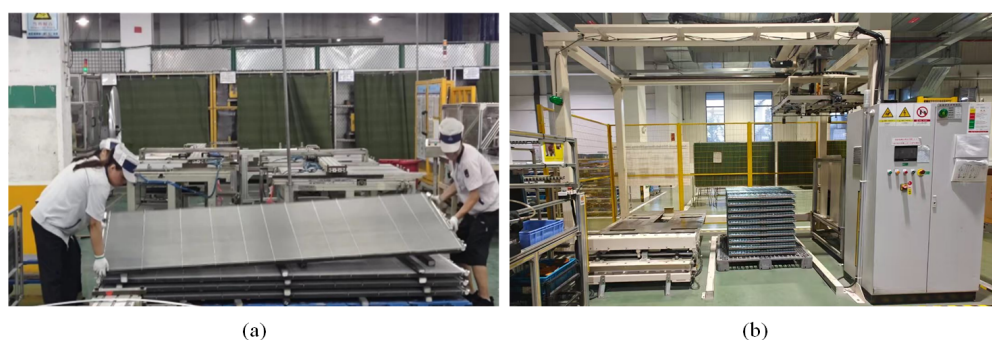
Figure 1. (a) manual loading; (b) automated loading.
