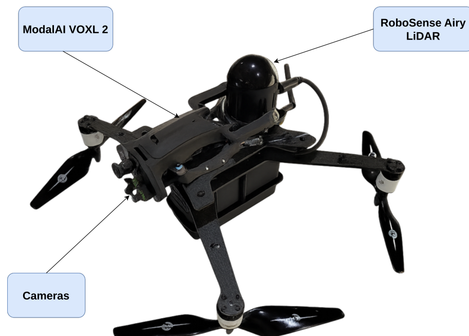
Figure 3. MANTIS UAV as flown in this work. The Airy LiDAR provides the input to the evaluated systems, the VOXL 2 runs them, and the tracking camera feeds the onboard VIO that serves as the reference at the warehouse.
