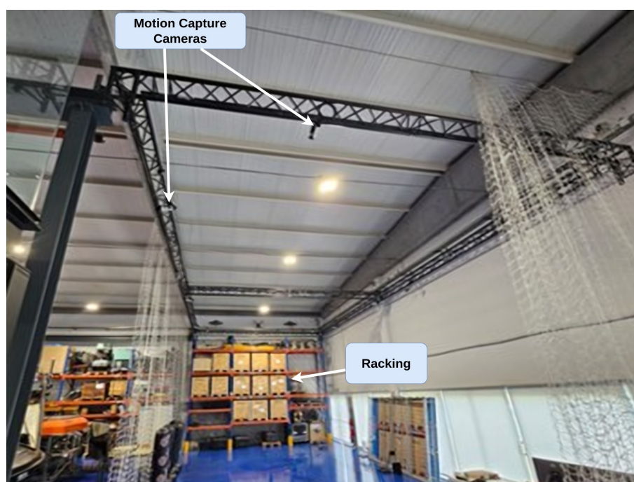
Figure 4. The laboratory site, where racking runs along one side only and the twelve-camera motion capture system provides the reference for the two recordings of the benchmark and the eight closed-loop flights.
