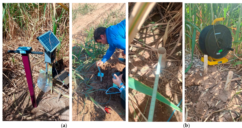
Figure 11. Field deployment and validation setup of the proposed sensing system: (a) soil-moisture sensing and field installation; (b) groundwater-level sensing and reference-measurement setup.
