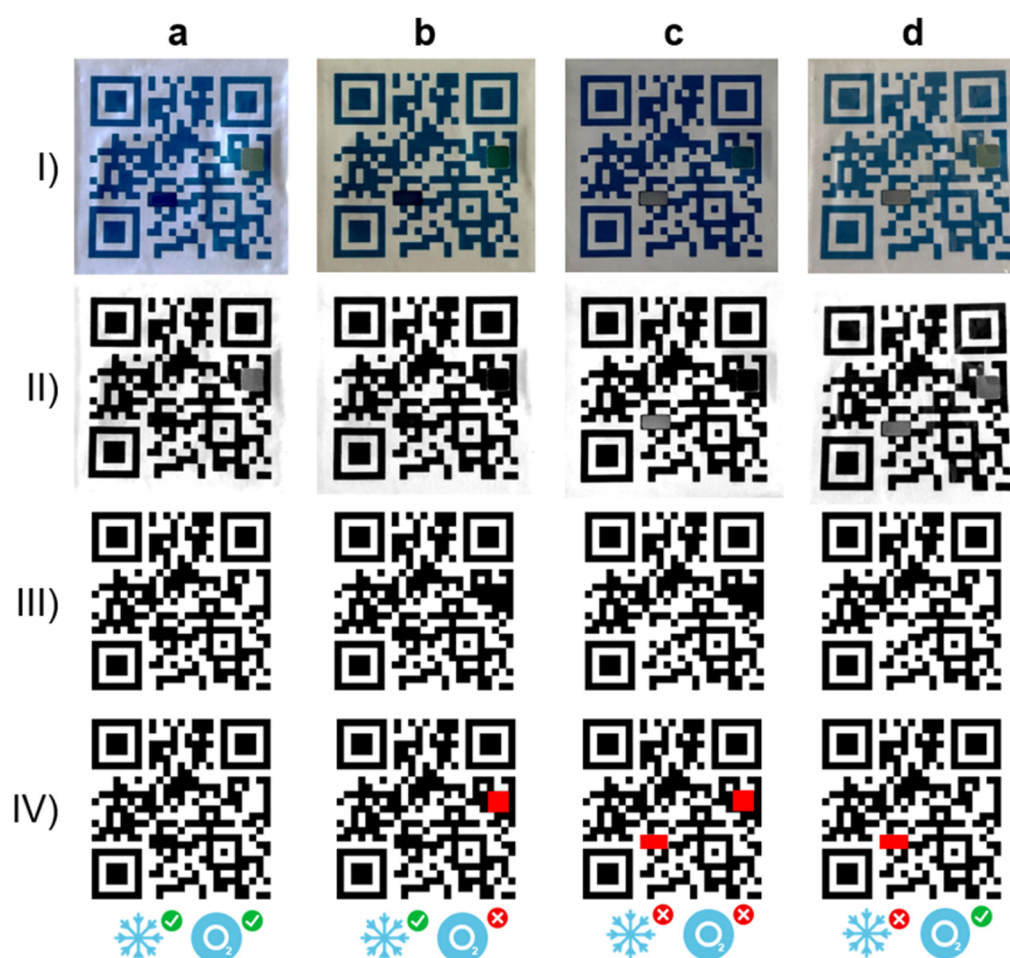
Figure 5. Full QR code sensor under the different conditions: (a) refrigerated and vacuum-sealed, (b) refrigerated and non-sealed, (c) non-refrigerated and non-sealed, and (d) non-refrigerated and vacuum-sealed. Different images correspond to (I) raw image under (no controlled light conditions), (II) W/B contrast-corrected image, (III) identified QR code, and (IV) module errors (in red) with respect to the expected QR code.
