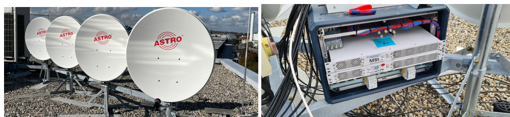
Figure 15. (Left) The satellite dishes pointed at a geostationary satellite. (Right) The SATCOM modems used for the combiner implementation and DVB demodulation. The modems are equipped with a 4-antenna RF front-end and an FPGA for real-time processing.
