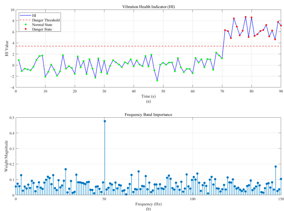
Figure 3. The proposed method applied to the performance of analog signal: (a) evolution of the Health Indicator (HI) over time; and (b) the optimized frequency weight vector |w^*| .
