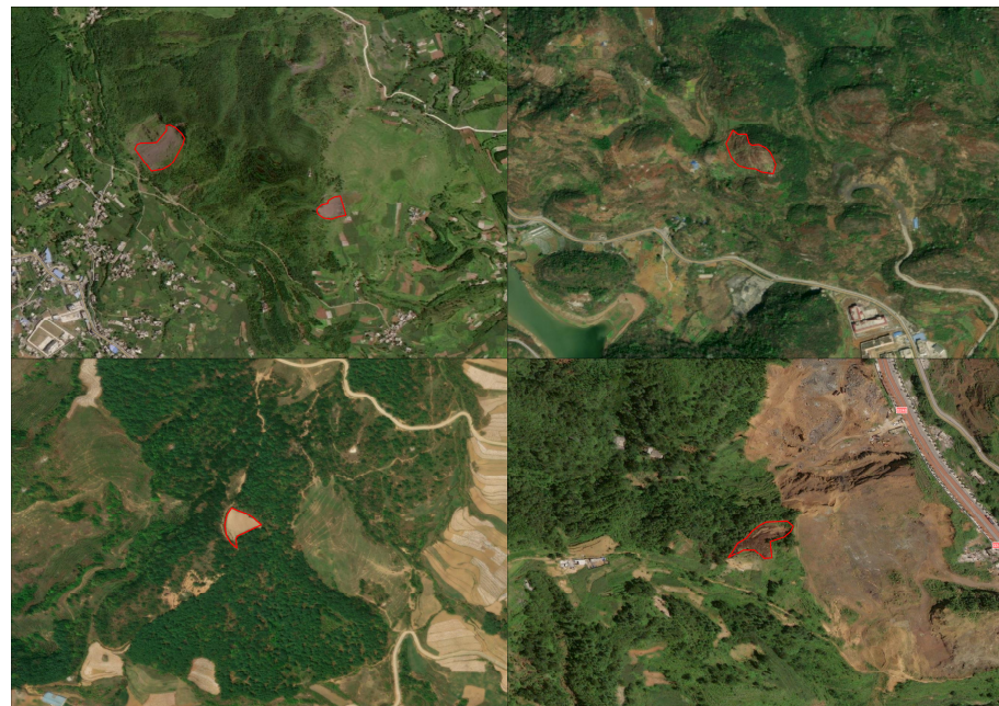
Figure 6. High-resolution optical images of four representative suspected landslide areas for validation of InSAR detection results (The red frames indicate the boundaries of the landslides).
