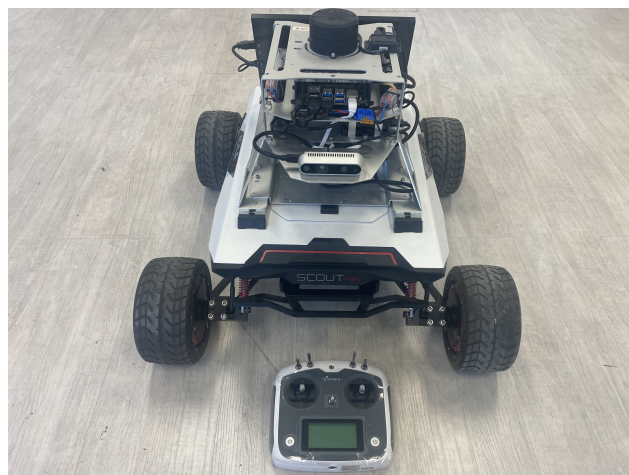
Figure 7. Experimental platform: Scout Mini equipped with a RealSense D435i camera and an embedded NVIDIA Jetson Xavier NX.
