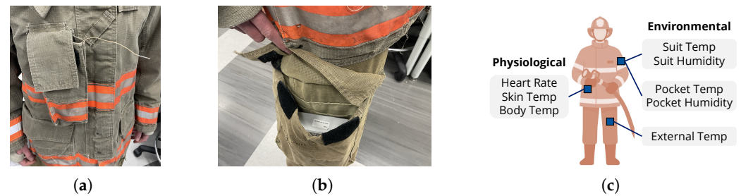
Figure 3. (a) Thermocouple probe in front pocket. (b) Data logging node worn in pant side pocket. (c) Firefighter sensors.
