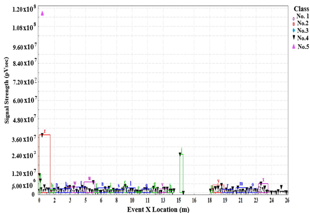
Figure 9. Scatter plot of signal strength as a function of location (beam length) for Beam No. 6 under static proof load. [Quantitative Annotation: 85% of zones active; Class 5 signal bursts detected exclusively in high-shear Zone 1, peaking at 1.15 \times 10^8 pVs].
