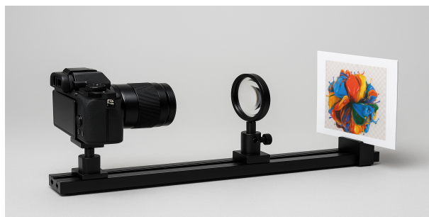
Figure 8. Optical acquisition device used to construct TexLensDB and CollensDB.
