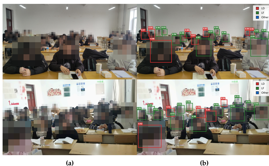
Figure 2. Representative classroom behavior detection results obtained using Cascade R-CNN from different fixed-camera viewpoints: (a) anonymized original classroom scenes and (b) corresponding behavior detection outputs.
