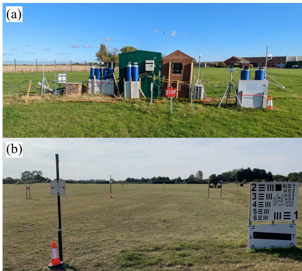
Figure 1. Testbed: (a) Testbed control building and installed cameras, LiDAR and radar. (b) View down the testbed as seen from sensors in (a); targets to left are LiDAR/radar with a camera resolution chart on the right.
