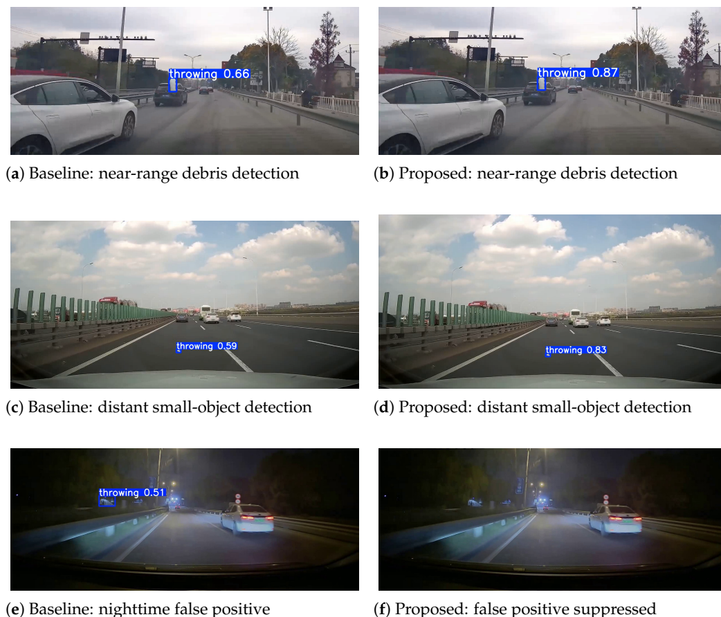
Figure 7. Qualitative comparison between the YOLOv8m baseline and the proposed MobileNetV4-YOLOv8m model. The first row shows near-range debris detection, the second row shows distant small-object detection, and the third row shows a nighttime reflective-interference case where the baseline produces a false positive while the proposed model suppresses it.
