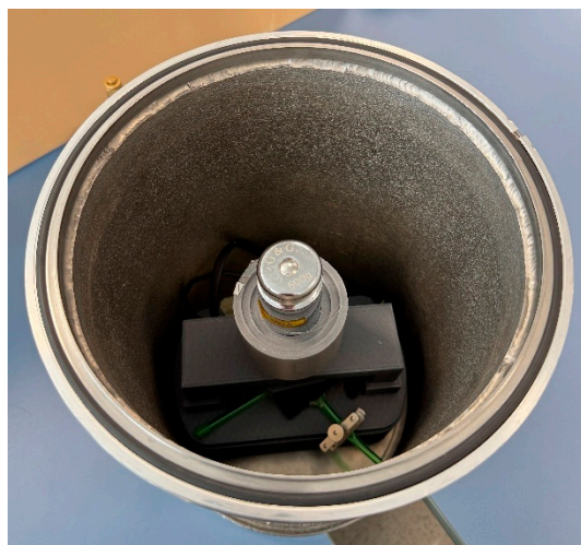
Figure 4. Top view of the experimental setup showing the pressure chamber without lid, the internal test rig with the air cushion in place, and a 500 g test weight applied to the indenter.
