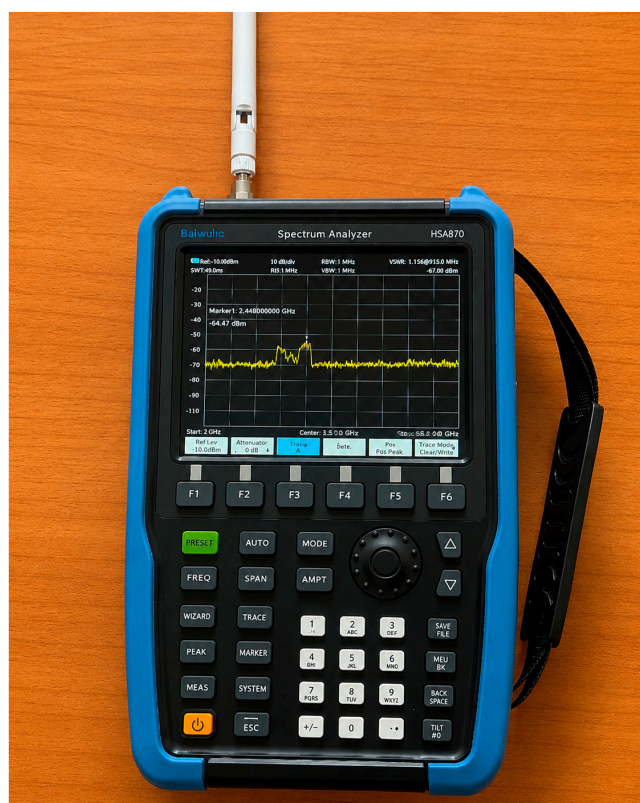
Figure 5. Experimental evaluation of the IEEE 802.11 wireless communication channel using the HSA870 spectrum analyzer.
