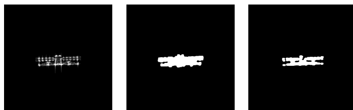
Figure 9. Failure case. (Left) Original ISAR image; (Middle) The mask when the AIL threshold is 16; (Right) The mask when the AIL threshold is 40.
