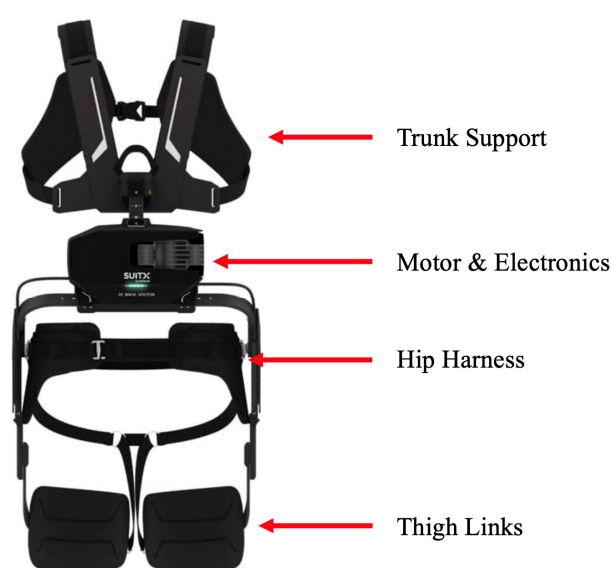
Figure 4. Schematic of the suitX exoskeleton used for evaluation.
