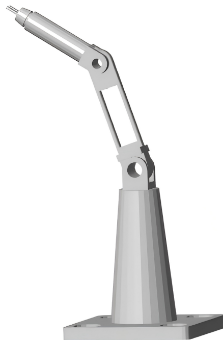
Figure 1. Schematic diagram of the 2-DOF robotic manipulator model.
