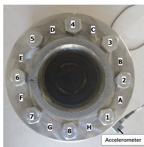
Figure 6. Schematic diagram of bolt positions and impact points.
