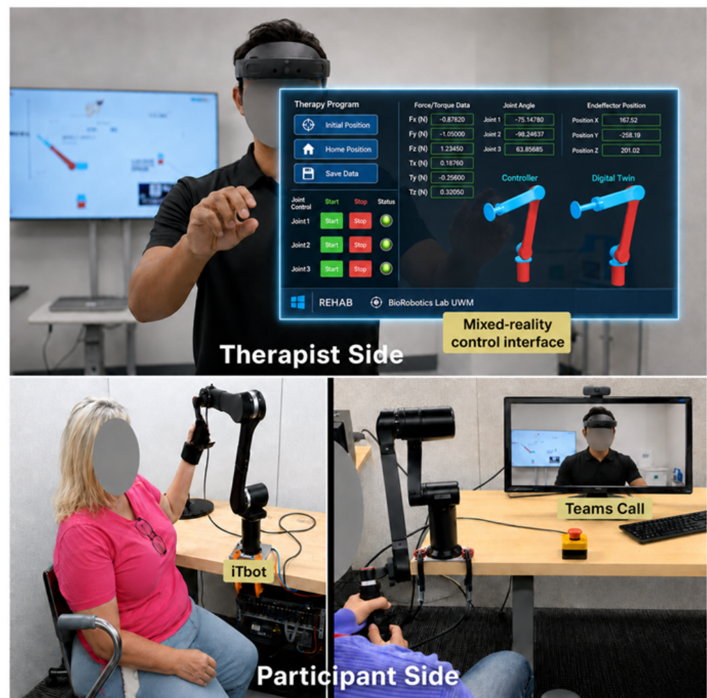
Figure 3. Two-station experimental setup simulating a telerehabilitation workflow. The upper panel shows the therapist side, where the occupational therapist uses Microsoft HoloLens 2 to interact with the MR-based control interface while monitoring the participant via a live Microsoft Teams video feed. The lower panel shows the participant side, where the stroke participant is seated at the desktop-mounted iTbot robot, grasps the wrist handle, and has access to the emergency stop switch.
