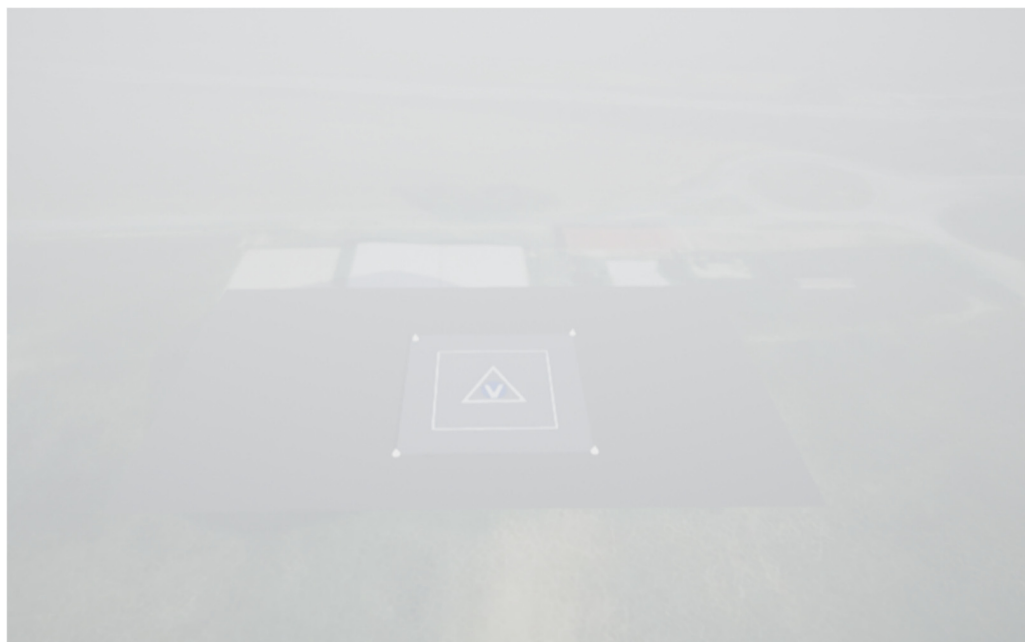
Figure 14. Forward-Looking (FL) camera image frame acquired through MATLAB® R2021a + Unreal Engine 4.23 (UE4) under low visibility. First usable in camera processing pipeline frame under dense fog ( R_{max,Cam} = 89 m).
